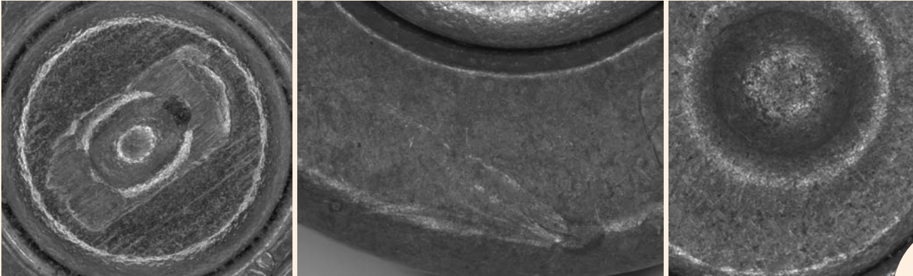
Same cartridge case markings in sector lighting
